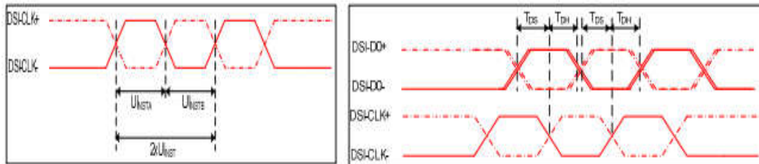
Figure 4 DSI clock channel timing
